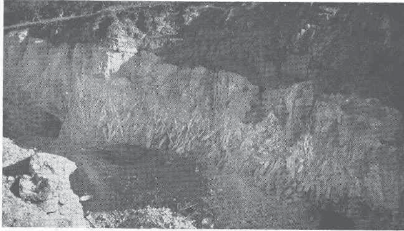
FIG. 1. Fringe-like aggregate of giant, lath-shaped spodumene crystals, Harding mine, New Mexico. The largest crystals are about 12 feet long. The quarry face here exposes the upper one-third of the thick, gently dipping pegmatite dike.
